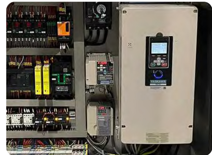
Soft start and stop of knives, bowl and extracting disc (optional) by mean of speed drives.
