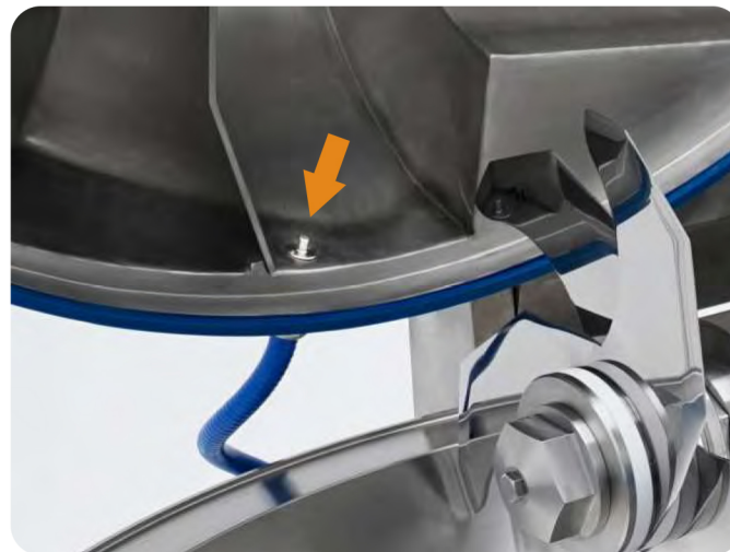
Fast and sensitive digital thermometer , with sensor extended into the internal cavity of the lid.
