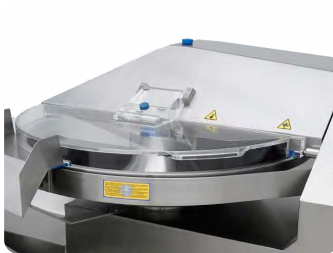
Transparent noise protection cover with automatic decrease of knife speed.
