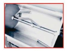
Pulse switch activates mixer when tilted for ease of unloading.
