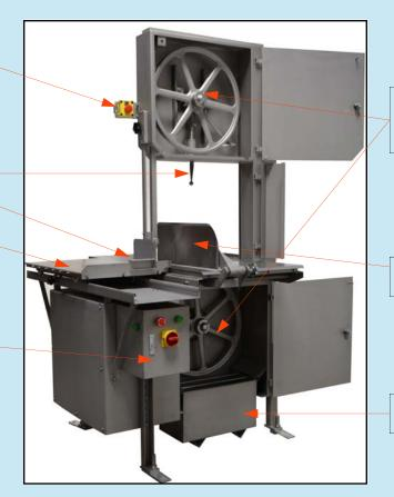
Stainless Steel Wheels w/ Sealed Bearings
