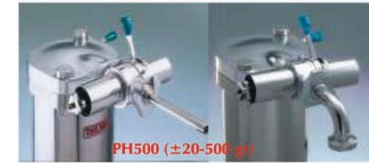
Option: Manual portioning device. Curved nozzle/horn with cutting valve to fill cans.
