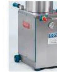
Wheels, pressure gauge, waterproof electric switchboard (mod. P).
