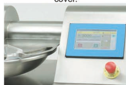
Emergency stop button.
